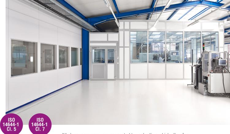
All clean room areas are connected to each other, which allow for production, cleaning and assembly in a contamination-free atmosphere. Quality control is fulfilled by specially trained personnel. Clean room manufactured products are prepared for transport in special double-welded packaging filled with class 5.0 nitrogen.
